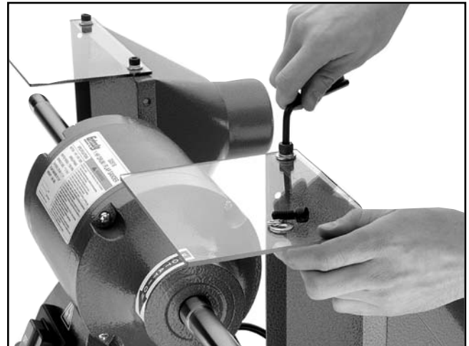
Figure 10. Attaching one of the acrylic eye shields.
